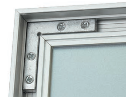
RFCA4 CORNER CONNECTOR 4 Connectors required per door 4 Fastening screws Minimum starting point for hinge is 78mm from middle line of corner connector.
