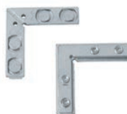
RFCA4 CORNER CONNECTOR 4 Connectors required per door 4 Fastening screws Minimum starting point for hinge is 78mm from middle line of corner connector.
